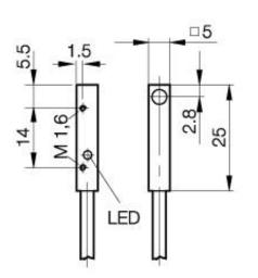
**Inductive Sensors** BES 516-3042-I02-C-PU-02 5 x 5 x 25 normally-closed Sn=0,8mm shielded
